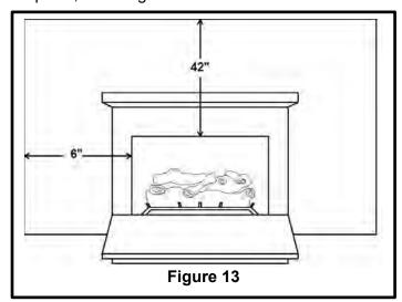
These dimensions are <u>MINIMUM CLEARANCES</u> to maintain when you install this burner system. The fireplace opening <u>MUST BE AT LEAST 6"</u> from any combustible sidewall. The ceiling <u>MUST BE AT LEAST 42"</u> from the top of the fireplace opening.
