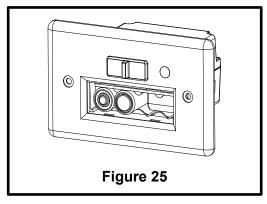
3. Set the same code combination, as used in the transmitter's code switches above, in the receiver, by using the receiver's code switches. Move the slide button to the "REMOTE" position (Figure 26) and place the receiver in front corner of the fireplace as far from the burner as possible.
